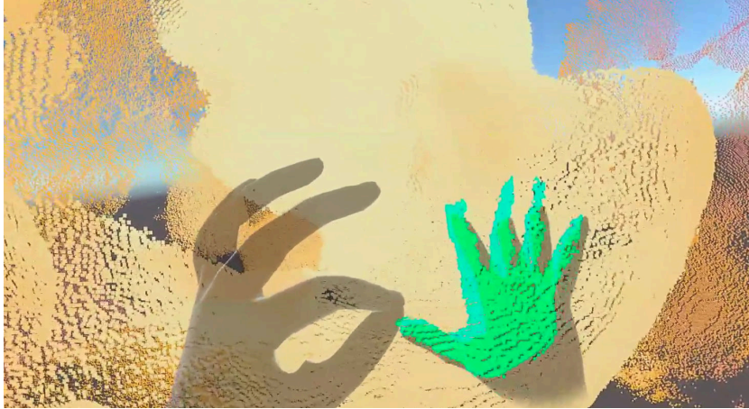
Figure 11: Brushing using the hand itself. Activated by pinching with the other hand.
