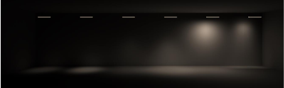
Figure 1 An empty room, illuminated by a diverse array of physically accurate lights. The configuration of these lights is achieved through the utilization of our web-based configurator, while the rendering process employs our texture baking and reverse path tracing approach in WebGL.
